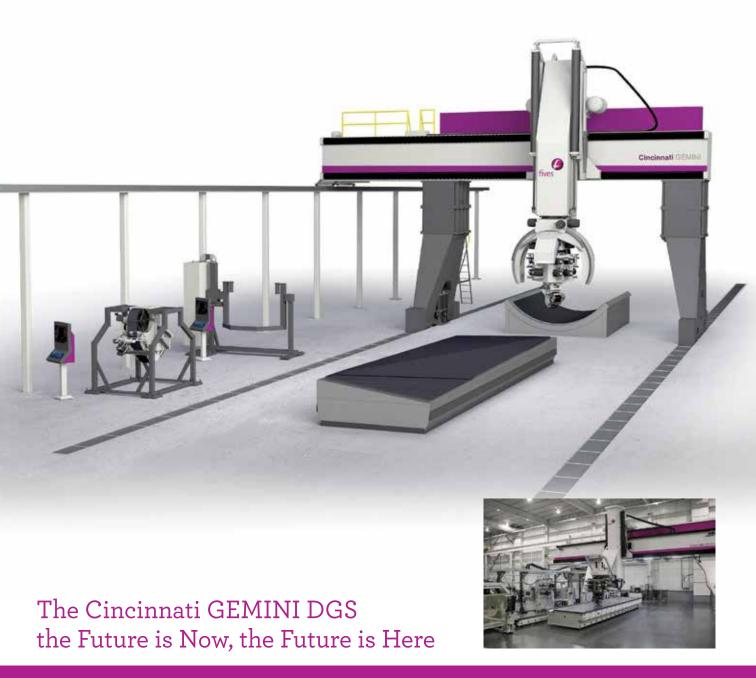
An industry FIRST, the Cincinnati GEMINI Dockable Gantry System combines Fiber Placement & Tape Laying dockable heads on a single platform
