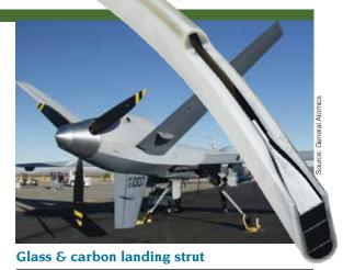
A fiberglass leaf spring made by LCRTM for the *Predator B MQ-9 Reaper* UAV. Its carbon fiber stiffener strengthens the attach point to the airframe (lower right).
