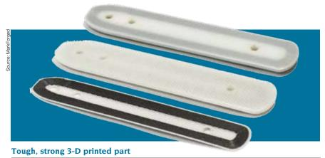
Two baseplates, like this produced by the Mark One machine, attach an aerowing to a race car. Essentially a sandwich construction, it features polyamide outer skins, continuous carbon reinforcement around the part perimeter, and a printed polyamide honeycomb core (center).
