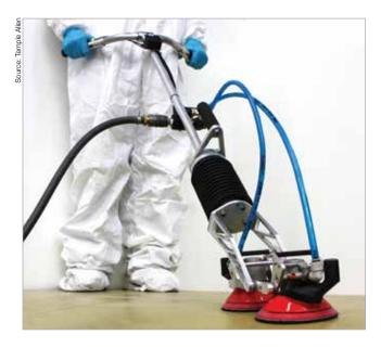
ing manual sanding, therefore, can damage the LSP, forcing replacement. The EMMA system employs a robotic arm, which in this case is designed to maintain uniform unit pressure and keep the sanding pads parallel with the blade surface. The worker operates the arm remotely, via control pad.
