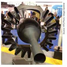
CMC jet engine exhaust cone
