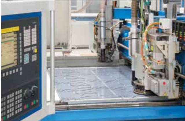
4 Blanks are cut on a high-speed, flatbed table cutter of proprietary design. Nesting software minimizes waste, and all waste can be recycled.
