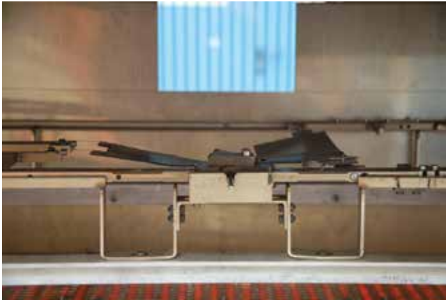
5 A closeup of a laminate blank as it is heated in one of two infrared ovens within the cell. Two ovens keeps the total cycle time lower; the heating step is the longest step, so two blanks can be heated while one is being shaped.
