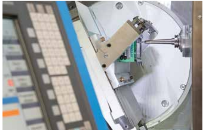
7 The trimming station cuts off beveled edges and ensures that the clip's final contour and shape are correct.
