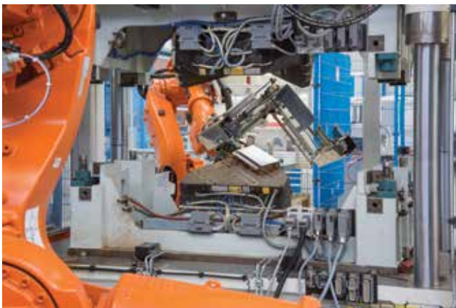
6 A clip is shown being robotically transferred from a tool in the 125-MT thermoforming press to the trimming station. The second, "slave" robot (visible in the foreground) transfers the correct tools to the press ahead of each heated blank that is transferred by the primary robot from the oven.
