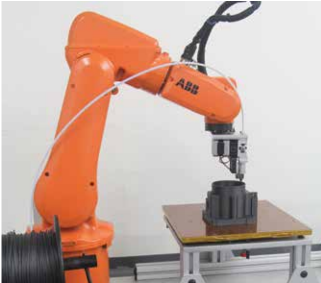
FIG. 4 RAMP adds z-axis fiber to 3D printing
