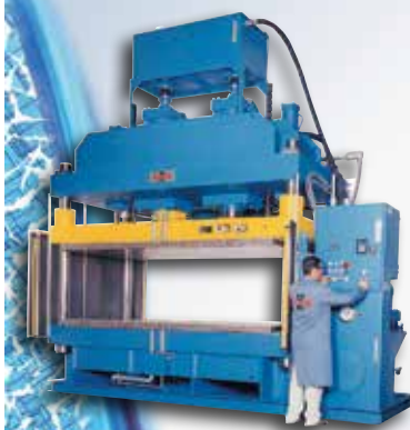
400 Tons Down-acting, 120" x 60" Platens
