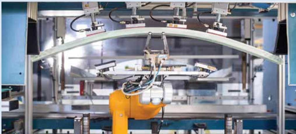
6 Finished prototype and production parts are NDT tested using automated ultrasound scanning.
