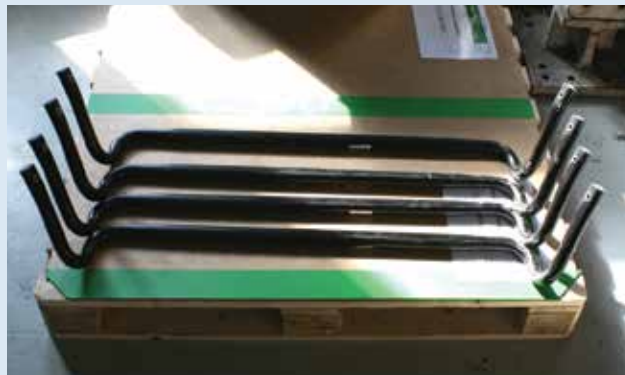
7 These pre-production CFRP stabilizer bars for the VW XLI passed all OEM-mandated tests in IFA Composite's extensive test center.
