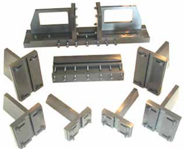
FIG. 2 A modular compression-after-impact test fixture for testing larger specimens.
