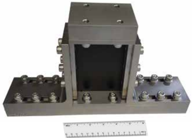
FIG. 1 An ASTM D 7137 compression-after-impact test fixture.
