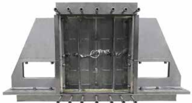
FIG. 3 Compression-after-impact testing of a stiffened composite panel.
