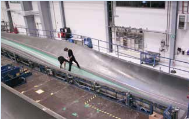
2 Mold release film is applied to the 45m blade's mold surface.
