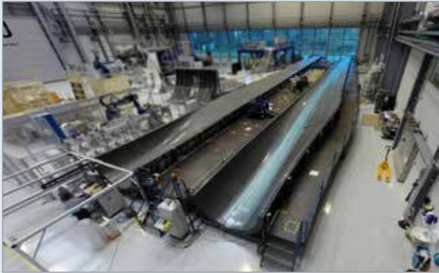
5 The resin infusion is completed in 46 minutes.
