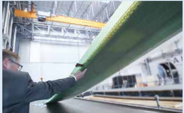
8 The finished spar cap is demolded.
