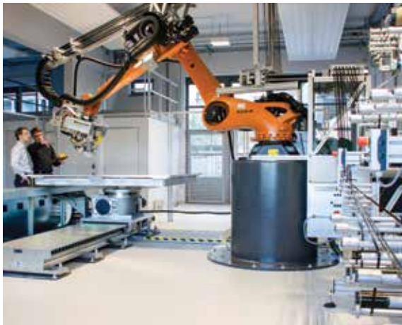
FIG. 3 Quick change head processes multiple materials quickly
