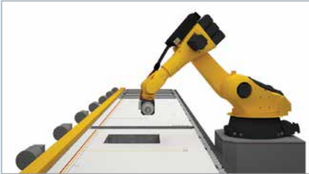
1 CAD files for this Pixel Haus kit were used to program CNC robots, which rout out window and door openings.
