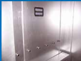
Interior Thermocouple Jack Panel & Vacuum Stubs
