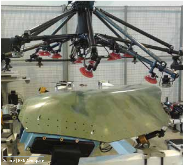
FIG. 4 CFRP elements for smaller, lighter fixtures
