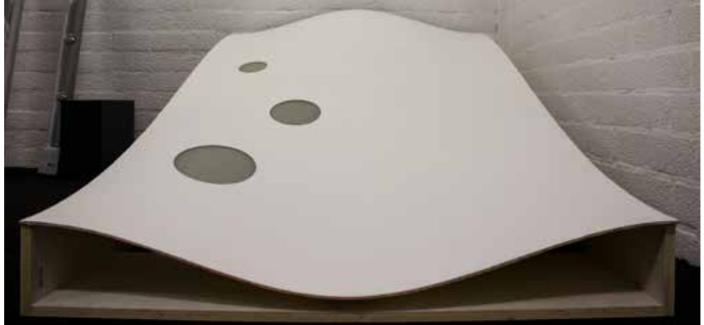
FIG. 2 One adaptive mold, myriad curved panels
